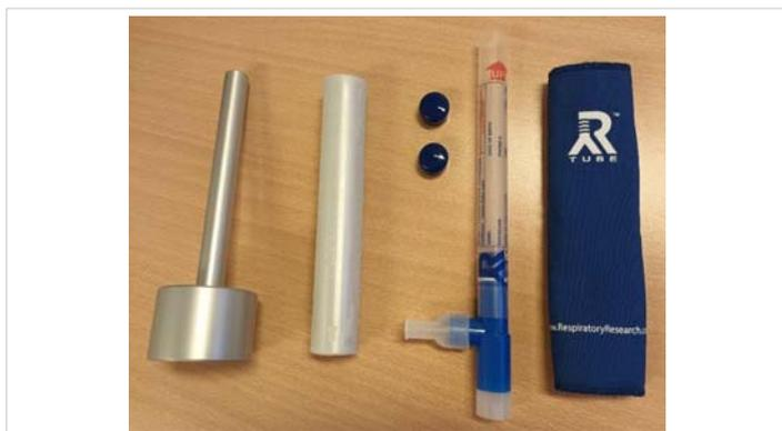
Figure 1: RTube (Respiratory Research, Austin, TX, USA). Right to left: Insulating cover, RTube – chamber, two endcaps, cooling sleeve and plunger.
