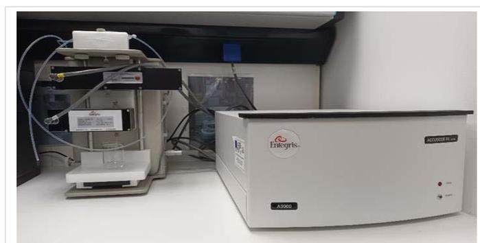
Figure 2: Accusizer FxNano (Particle Sizing Systems Inc., Port Richey, FL, USA). The syringe with the tubes to pump the sample and the sensors (black squares) are on the left side of the figure and the counter is on the right.
